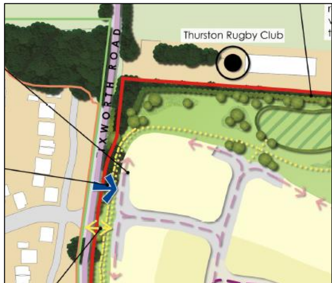
Figure 4: Indicative emergency vehicle access
